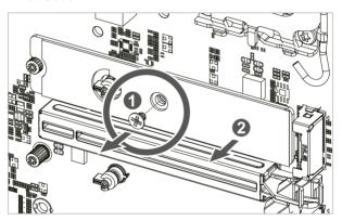
※ Depending on the design of the motherboard, be sure to replace the standoff after removing the M.2 heatsink to install the SSD.
