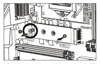
※ Be sure to replace the standoff after removing the M.2 heatsink in order to install the SSD. 主機板的M.2散熱片移除後須再將螺柱鎖回才能安裝SSD。
