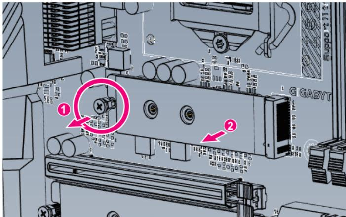
※ Be sure to replace the standoff after removing the M.2 heatsink in order to install the SSD.
