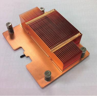
A rectangular copper heat sink with a dense grid of vertical fins. It is mounted on a copper base plate with four screws. A small black component is visible on the bottom edge. |
