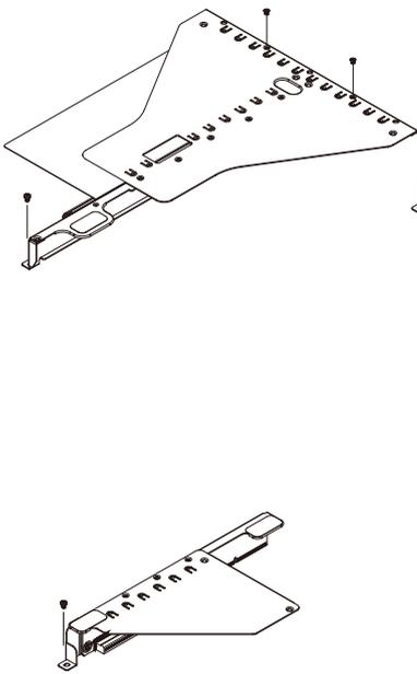
3. Attach the support brackets to GPU cards and secure the brackets with screws.
