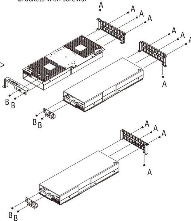
4. Install the GPU card to system and secure the card with screws.
