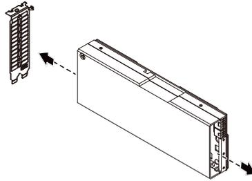
2. Remove the securing screw on the riser bracket and lift up the it out of system.
