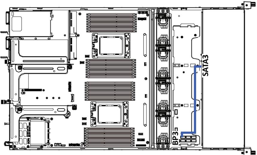
Expander to HDD Backplane Board Cable #4
