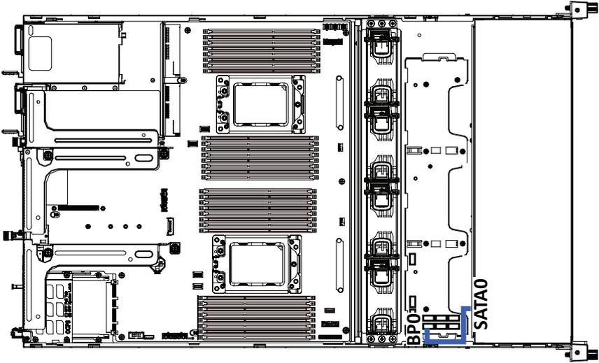
Expander to HDD Backplane Board Cable #1
