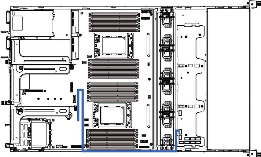
Expander to HDD Backplane Board Cable #0
