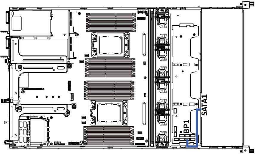
Expander to HDD Backplane Board Cable #2
