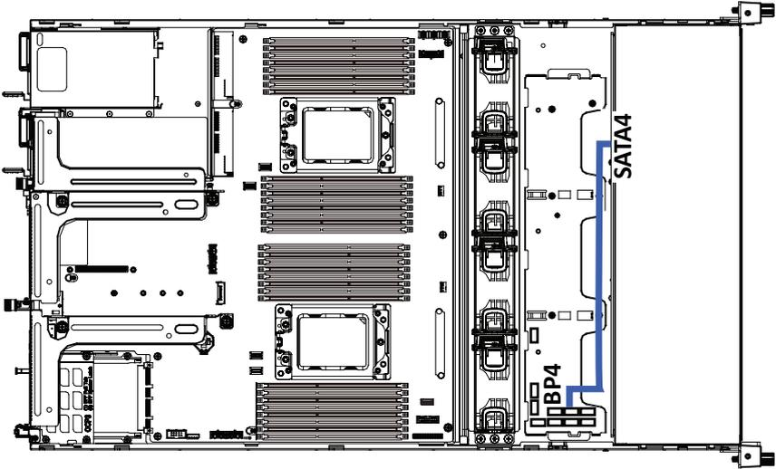
Expander to Rear HDD Backplane Board Cable #5
