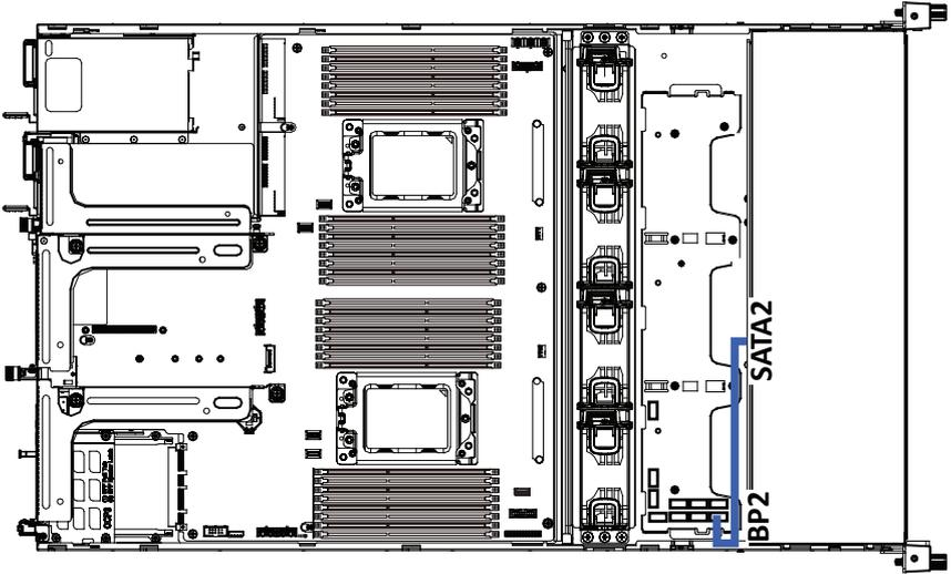
Expander to HDD Backplane Board Cable #3
