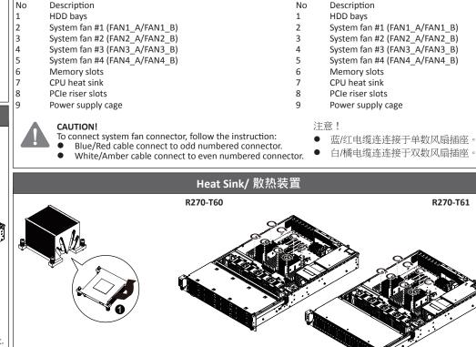
Remove fan duct before installing the CPU heat sinks.
