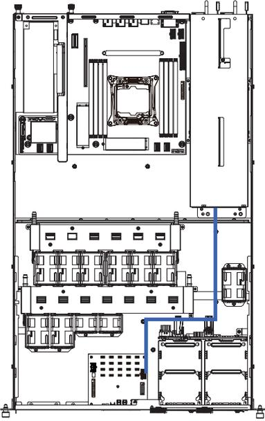
HDD Back Plane Board Power Cable
