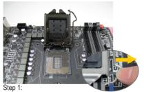
Gently press the CPU socket lever handle down and away from the socket with your finger. Then completely lift the CPU socket lever and the metal load plate will be lifted as well.
