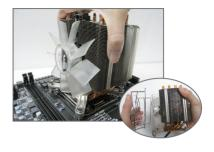
Step 2: Place the cooler atop the CPU, aligning the four mounting screws with the mounting holes on the ILM. (If your cooler has a fan grill which may cause interference when you tighten the screws, remove it first and replace it after tightening the screws.)
