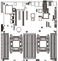
10) SW\_RAID (Intel/LSI Software RAID Key Header)
