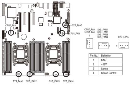
Be sure to connect fan cables to the fan headers to prevent your CPU and system from overheating. Overheating may result in damage to the CPU or the system may hang.
