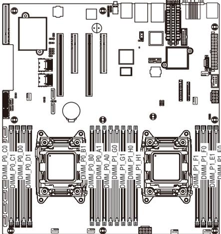
Due to CPU limitations, read the following guidelines before installing the memory in Four Channel mode.
