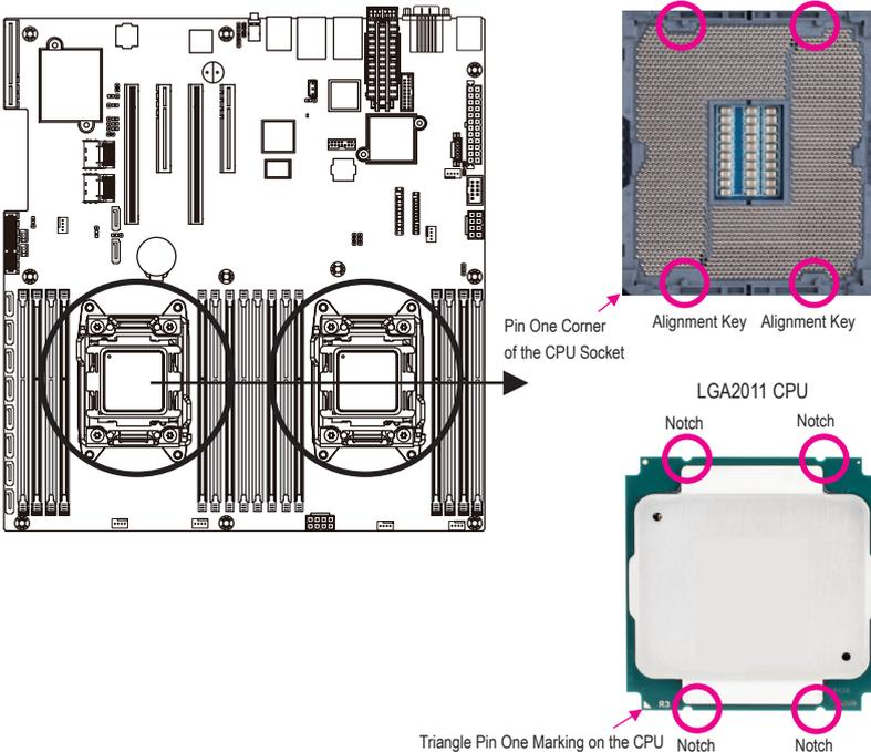
B. Follow the steps below to correctly install the CPU into the motherboard CPU socket.
