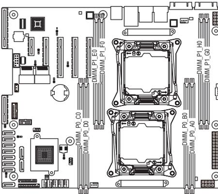
Due to CPU limitations, read the following guidelines before installing the memory in Four Channel mode.
