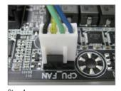
Step 4: Finally, attach the power connector of the CPU cooler to the CPU fan header (CPU\_FAN) on the motherboard
