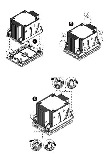
To install/remove the Intel heatsink use a T30-Lobe screwdriver or drill bit with a screw torque of 8.0 +/- 0.5kgf\*cm
