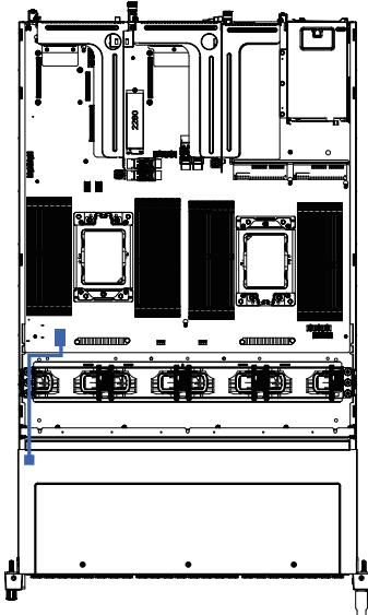
**On board SATA to HDD Back Plane Board Mini-SAS HD RAID Card Cable
