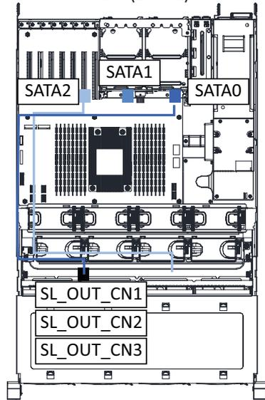
Rear HDD Back Plane Board Signal Cable
