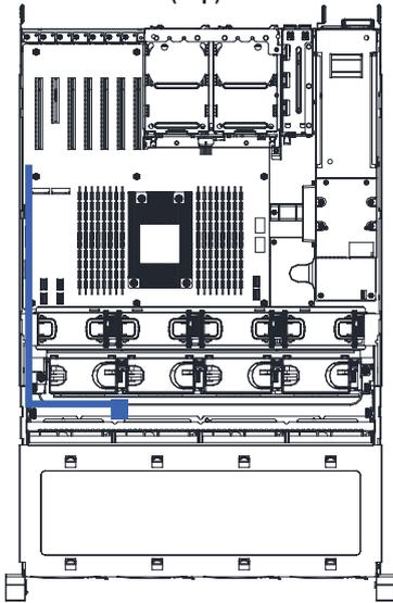
Front HDD BPB to Rear HDD BPB SAS HDD
