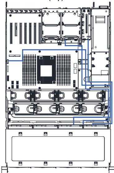
Rear HDD Back Plane Board Signal Cable
