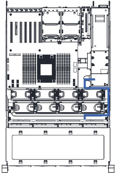
**Rear HDD Back Plane Board Power Cable**
