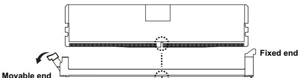
2. Hold it with both hands, insert the memory module into the movable end first, and then insert the memory module into the fixed end.
