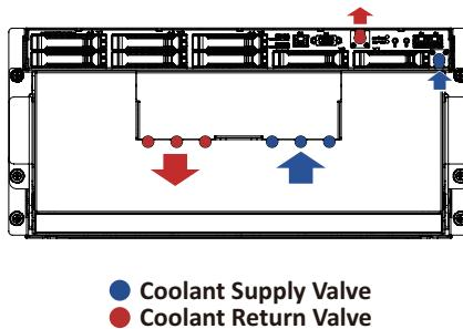
The flow of the CPU coolant is shown below:
