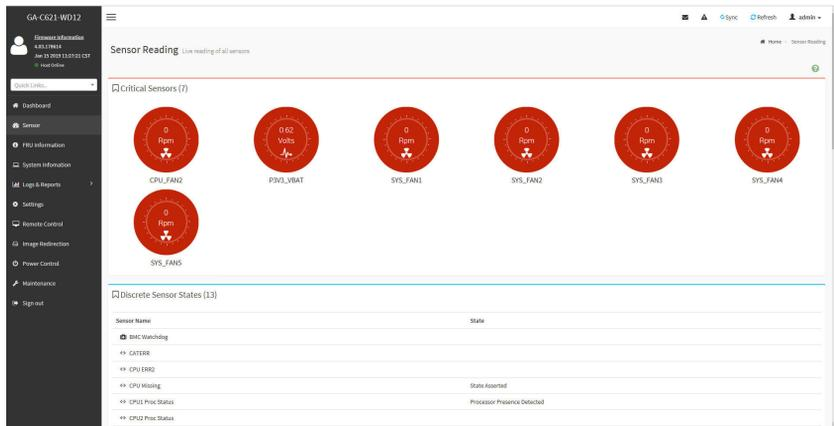
On this page, details for all the available sensors e.g. Name, Type, Status, Current Reading and Behavior are displayed. The sensor readings are available for Temperature, Fan, Watchdog and Voltage Sensors as well as for supported Discrete Sensors. This page will refresh automatically with the latest data retrieved from the database. Please note that there may be some delay in retrieving this live data. Sensors are organized by their Type and State (Critical, Discrete, Normal and Disabled).
