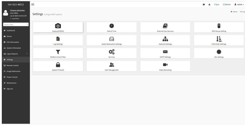
This page allows you to configure BMC options. The options are: Captured BSOD, Date & Time, External User Services, KVM Mouse Setting, Log Settings, Media Redirection Settings, Network Settings, PAM Order Settings, Platform Event Filter, Services, SMTP Settings, SSL Settings, System Firewall, User Management, and Video Recording.
