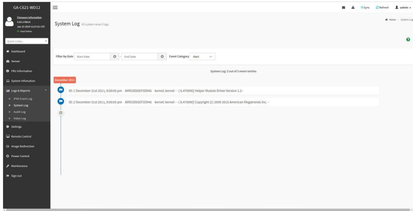
This page displays logs of system events for this device (if the options have been configured). **Note:** Logs must be configured under "Settings/Log Settings/Advanced Log Settings" to display any entries. Filtering options are also available for this and all logs in this section.
