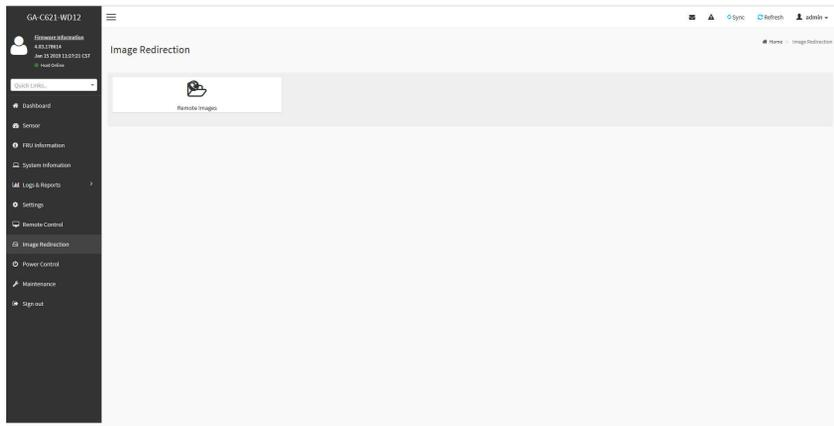
The displayed table shows remote images available to the BMC. You can start redirection or clear the images from here. Up to 4 images can be added for each image type, depending on your configuration.
