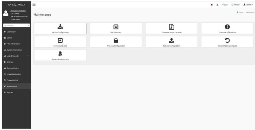
This page allows you to configure BMC options. The options are Backup Configuration, BMC Recovery, Firmware Image Location, Firmware Information, Firmware Update, Preserve Configuration, Restore Configuration, Restore Factory Defaults, and System Administrator.
