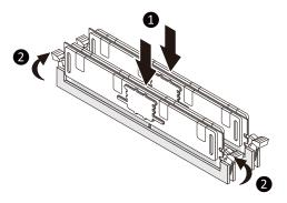
Note: When installing the memory in Channel 1 or Channel 4, make sure to begin with DIMM-A1 or DIMM-D1, or the system will not boot properly.
