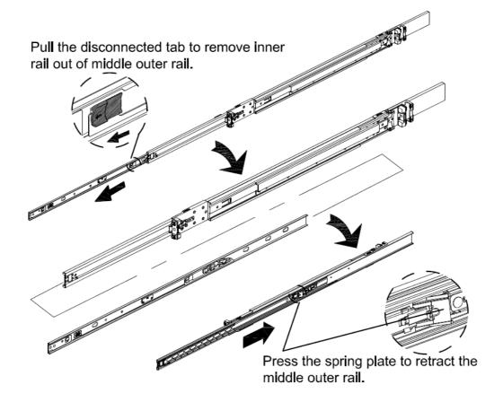
5. Install inner rail to both side of chassis.
