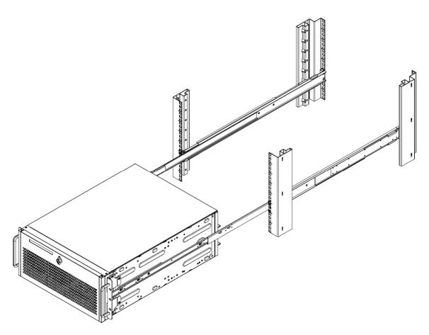
7-3 Use M5 screws to lock the chassis to the rack.
