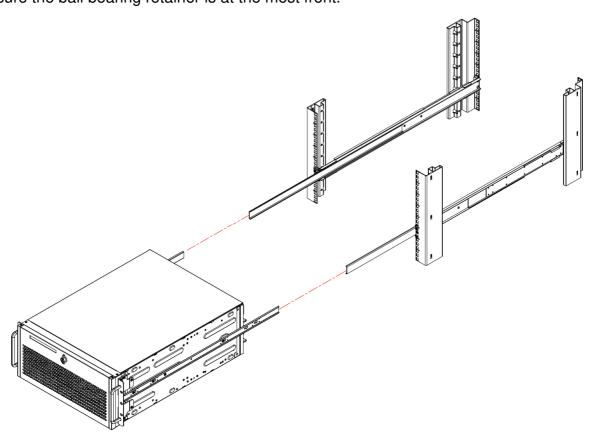
7-2 Installing chassis into middle outer rails, when the chassis is locked, pull the released tab on the inner rail and proceed to pull the chassis into rack.
