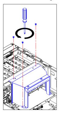
3. Lift the duct out of the chassis.
