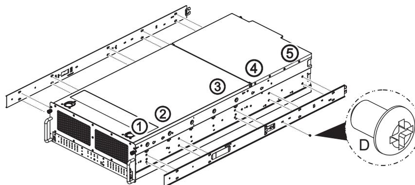
4) Insert the chassis to complete the installation.
