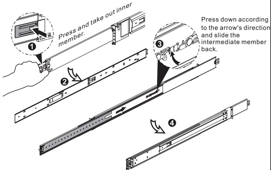
2) Install the inner member onto the chassis.
