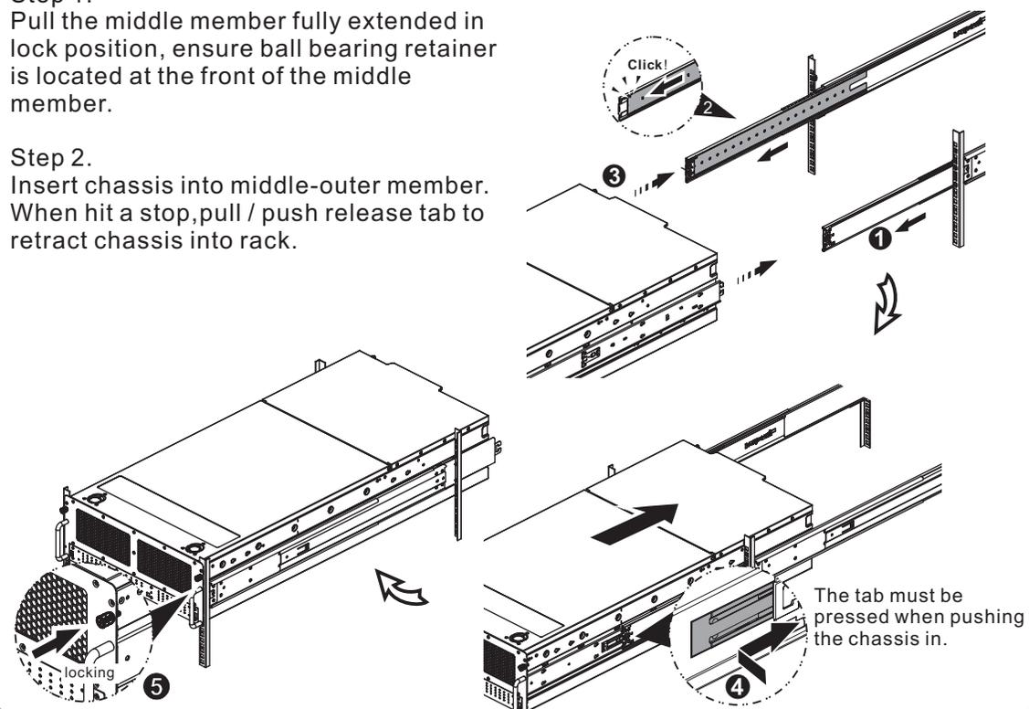
3) Attach the outer member/bracket to the rack.
