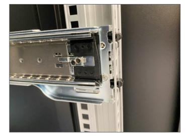
The front side and rear side assembly methods are the same. Attach the mounting bracket to the rack posts. Then lock on and push
