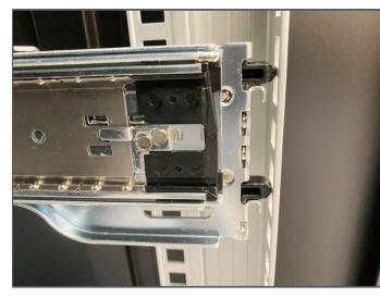
Position the slide rail assembly in your rack and attach the mounting bracket to the rack posts. Then lock on and push down.
