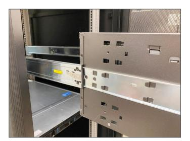
2 Align the front section of the W42G-P08R with the rail assembly and insert it. and right slides simultaneously to prevent any stuck during the insert process.)
