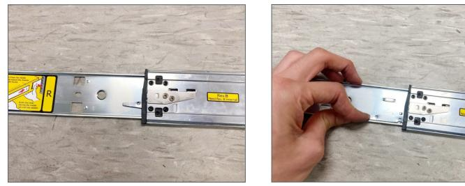
**3** Push the latch between the front and middle section of the rail assembly, then simultaneously withdraw the front section from slide rail assembly.
