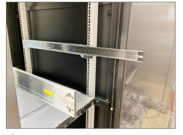
1 Pull out the slide rail assembly on your rack until it stops.
