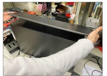
Position the front section against the W42G-P08R, and make sure the mounting holes on the front section are aligned with the locating pins on the side of the W42G-P08R. Assemble the front section onto the W42G-P08R and pull back to lock on. (NOTE: Make sure the below fixed bracket is
