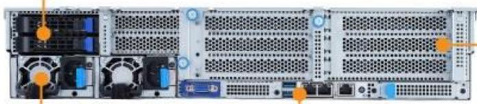
Dual 1200W redundant power supply
