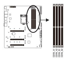
▶ Recommanded Dual Channel Memory Configuration:
