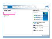
The **Status** item on the left of the screen displays the rebuild progress. After the RAID 1 volume rebuilding, the **Status** will display as **Normal**.
