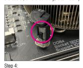
You should hear a "click" when pushing down each push pin. Check that the Male and Female push pins are joined closely.
