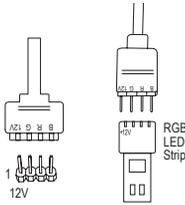
Connect one end of the RGB LED strip extension cable to the header and the other end to your RGB LED strip. The black wire (marked with a triangle on the plug) of the extension cable must be connected to Pin 1 (12V) of this header. The 12V pin (marked with an arrow) on the other end of the extension cable must be lined up with the 12V of the LED strip. Be careful with the connection orientation of the LED strip; incorrect connection may lead to the damage of the LED strip.
