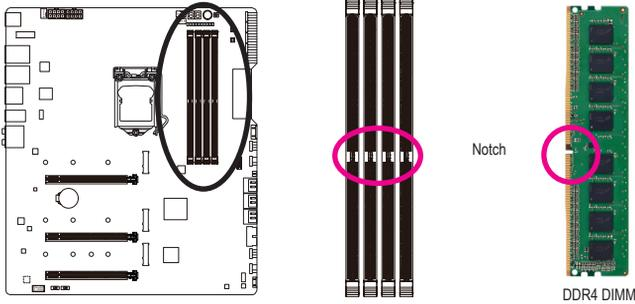
A DDR4 memory module has a notch, so it can only fit in one direction. Follow the steps below to correctly install your memory modules in the memory sockets.
