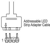
Connect one end of the included addressable LED strip adapter cable to this header and the other end to your addressable LED strip. The power pin (marked with a triangle on the plug) of the LED strip must be connected to Pin 1 of the addressable LED strip header. Incorrect connection may lead to the damage of the LED strip.
