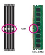
A DDR4 memory module has a notch, so it can only fit in one direction. Follow the steps below to correctly install your memory modules in the memory sockets.
