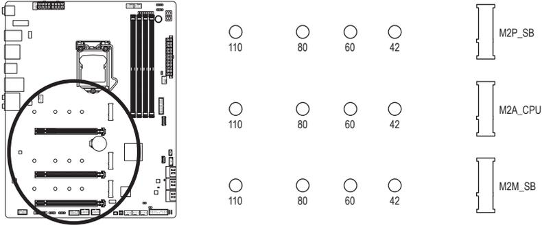
Follow the steps below to correctly install an M.2 SSD in the M.2 connector.
