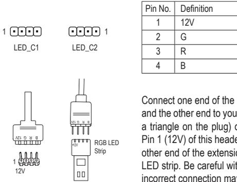
Connect one end of the RGB LED strip extension cable to the header and the other end to your RGB LED strip. The black wire (marked with a triangle on the plug) of the extension cable must be connected to Pin 1 (12V) of this header. The 12V pin (marked with an arrow) on the other end of the extension cable must be lined up with the 12V of the LED strip. Be careful with the connection orientation of the LED strip; incorrect connection may lead to the damage of the LED strip.
