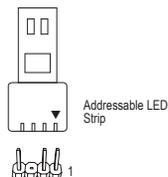
Connect your addressable LED strip to the header. The power pin (marked with a triangle on the plug) of the LED strip must be connected to Pin 1 of the addressable LED strip header. Incorrect connection may lead to the damage of the LED strip.
