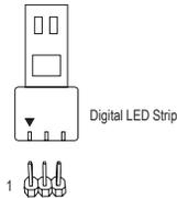
Connect your digital LED strip to the header. There are 12V and 5V digital LED strips. Be sure to verify the voltage requirements of your digital LED strip and set the DLED\_V\_SW1 and DLED\_V\_SW2 jumpers accordingly. The power pin (marked with a triangle on the plug) of the LED strip must be connected to Pin 1 of the digital LED strip header. Incorrect connection may lead to the damage of the LED strip.
