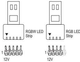
Connect your RGB (RGBW) LED strip to the header. The power pin (marked with a triangle on the plug) of the LED strip must be connected to Pin 1 (12V) of this header. Incorrect connection may lead to the damage of the LED strip.
