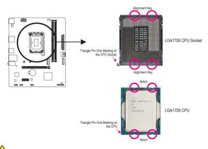
Do not remove the CPU socket cover before inserting the CPU. It may pop off from the load plate automatically after you insert the CPU and close the load plate.
