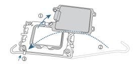
Do not force to engage the CPU socket locking lever when the CPU is not installed correctly as this would damage the CPU and CPU socket.
