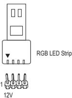
Connect your RGB LED strip to the header. The power pin (marked with a triangle on the plug) of the LED strip must be connected to Pin 1 (12V) of this header. Incorrect connection may lead to the damage of the LED strip.
