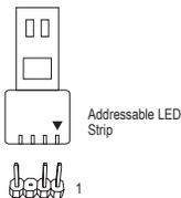
Connect your addressable LED strip to the header. The power pin (marked with a triangle on the plug) of the LED strip must be connected to Pin 1 of the addressable LED strip header. Incorrect connection may lead to the damage of the LED strip.
