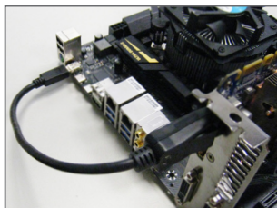
Step 1: Connect your Mini-DisplayPort cable (purchased separately) from the graphics card to the Mini-DisplayPort In on the back panel.
