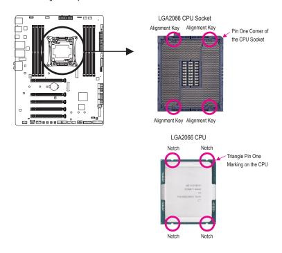
B. Follow the steps below to correctly install the CPU into the motherboard CPU socket.
