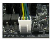
Step 4: Finally, attach the power connector of the CPU cooler to the CPU fan header (CPU\_FAN) on the motherboard.
