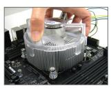
Step 2: Place the cooler atop the CPU, aligning the four mounting screws with the mounting holes on the ILM.
