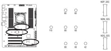
Follow the steps below to correctly install an M.2 SSD in the M.2 connector. The following steps demonstrate how to install an M.2 SSD in the M2Q\_32G connector.
