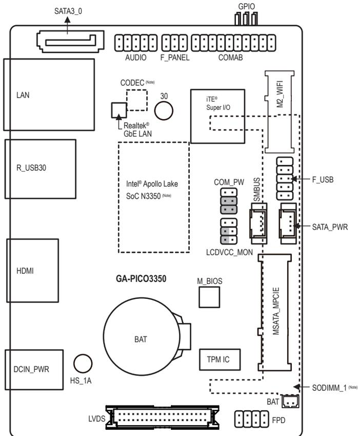
(Note) This chip/connector is on the back of the motherboard.
