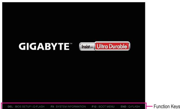
There are two different BIOS modes as follows and you can use the <F2> key to switch between the two modes. The Classic Setup mode provides detailed BIOS settings. You can press the arrow keys on your keyboard to move among the items and press <Enter> to accept or enter a sub-menu. Or you can use your mouse to select the item you want.
