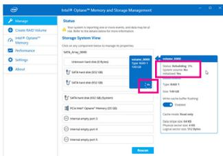
The **Status** item on the right of the screen displays the rebuild progress. After the RAID 1 volume rebuilding, the **Status** will display as **Normal**.
