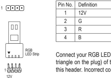
Connect your RGB LED strip to the header. The power pin (marked with a triangle on the plug) of the LED strip must be connected to Pin 1 (12V) of this header. Incorrect connection may lead to the damage of the LED strip.
