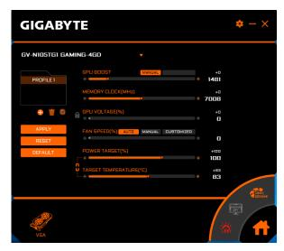
Users could also choose CUSTOMIZED for fan setting, and move the white dots on the line chart to adjust fan speed and temperature.
