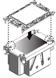
2 When installing the heatsink to CPU, use a T30 Lobe screwdriver to tighten 4 captive nuts in sequence as 1-4. The screw tightening torque:  $8 \pm 0.5$  kgf-cm.
