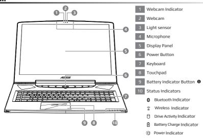
Press the right button of touchpad to check the remaining battery power. Right click to show the remaining power percentage.
