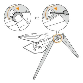
**Note:** You can either use a coin or a small flathead screwdriver to tighten the screw.
