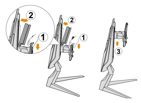
3. Place the monitor on the package cushion or a flat surface, with screen facing down. Tear apart the EPE bag, install the stand on the rear side of the monitor. Then you can take the monitor from the lower EPS foam by holding the stand arm. Carefully lift the monitor. Place it upright on a table.
