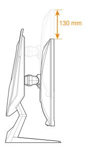
**Note:** Before making the height adjustment, make sure you have removed the safety plate from the stand.
