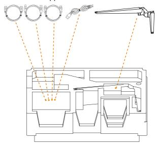
**4.** Remove the upper EPS foam. Then you can remove the stand from the lower EPS foam.
