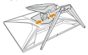
3. Pull down the stand slightly to disengage the hooks. Then remove the stand.
