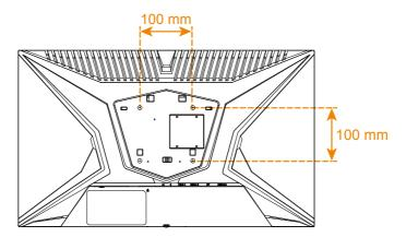
**Note:** To mount the monitor on the wall, refer to the installation guide that is included in the wall-mount bracket kit.
