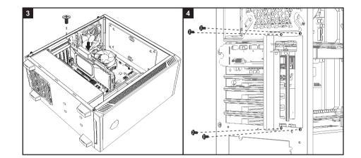
Install the additional system fan(not included) 安裝系統風扇 (額外添購) / 安装系统风扇 (额外添购)
