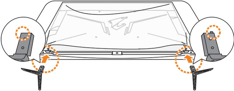
3. Secure the monitor bases with the four screws.
