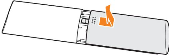
2. Insert two AAA batteries into the battery compartment. Ensure that the batteries are inserted with the correct polarity.
