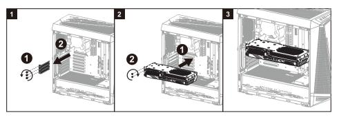
4.2 Vertical VGA card installation (requires optional PCI-E x16 riser cable) 垂直式顯示卡安裝 (需額外添購PCIE延伸線) / 垂直式显卡安装(需额外添购PCIE延伸线)
