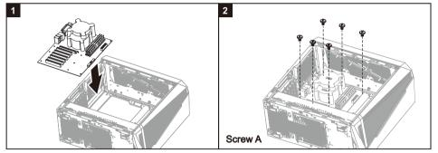
\*The quantity of standoff 6.5mm depends on motherboard's type. \*銅柱所需數量取決於主機板類型 \*铜柱所需数量取决于主机板类型
