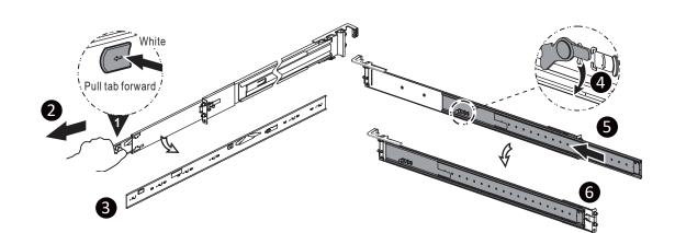
Install the outer member/bracket assembly to the frame. 3)
